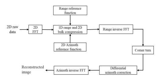
Figure 5 The diagram of Stolt interpolation algorithm processing.
