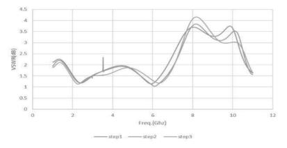
Figure 4: The comparison between VSWRs of all three antennas
