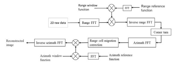
Figure 4. A flow diagram of the Range-Doppler algorithm.
