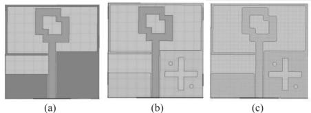
**Figure 2:** a) The initial design of the proposed antenna b) Micro-strip antenna with plus and circular shaped cuts c)The proposed antenna
