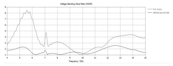
Figure 5 The designed antenna VSWR comparison with the result of the same design before the ground slots refining.
