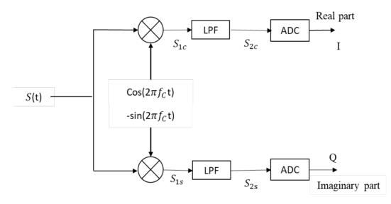
Figure 2 Quadrature demodulator
