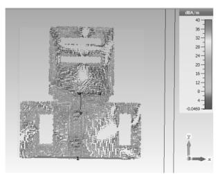
Figure 10 The Designed antenna Surface current distribution
