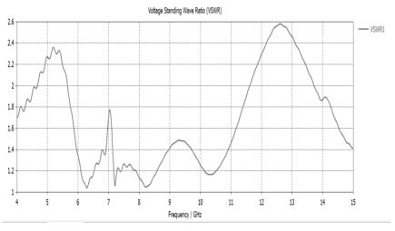
Figure 6 The Designed antenna VSWR
