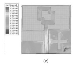
Figure 6: Surface current distribution of the a) initial design b) second design c) proposed antenna
