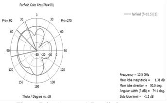
Figure 7 the Antenna 1-D radiation pattern
