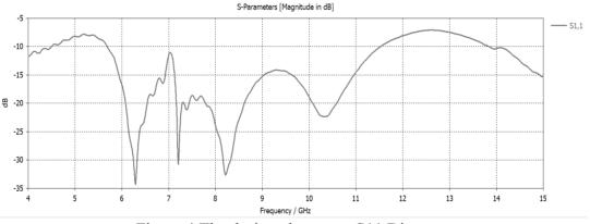
Figure 4 The designed antenna S11 Diagram
