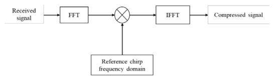
Figure 3 Block diagram of DFT-based pulse compression
