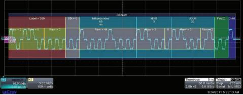
Figrue 1. An ARINC 429 Word, viewed as a signal, with overlaid decoding
