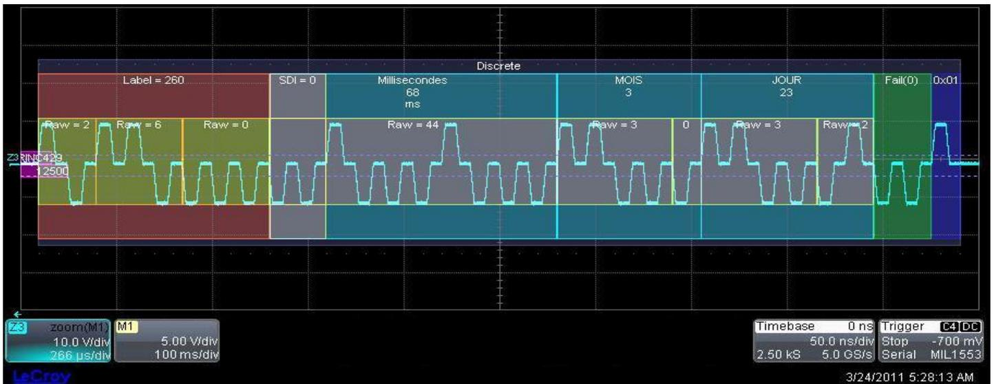
Figure 1. An ARINC 429 Word, viewed as a signal, with overlaid decoding
