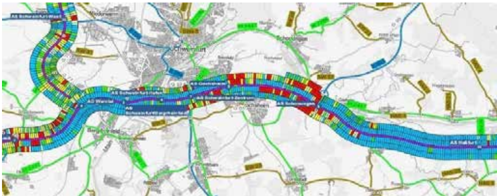
Fig.1. Dataset (4,839 road sections, each 100 meters long) describing road conditions and traffic density on the A70 road plan [1].
