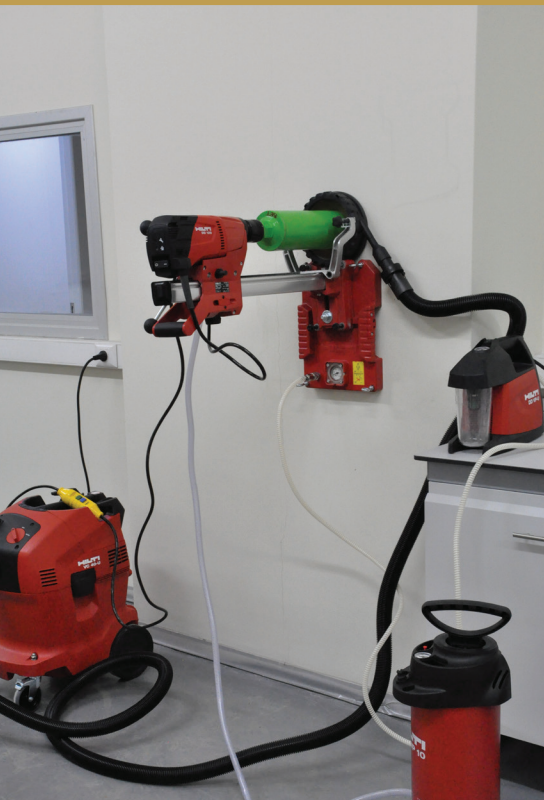
Vakum Tabanlı Karot Alma Sistemi Core Vacuum-Based Making System
